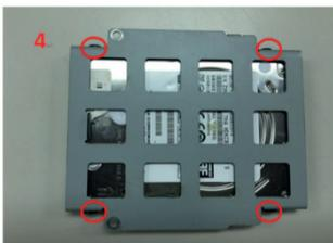
5. Remove the hard drive from the hard drive bracket
