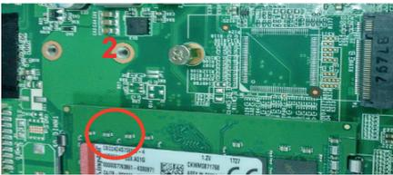
3. Install the M.2 2242 SSD into the socket
