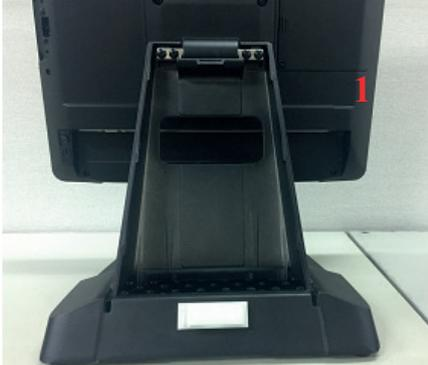
2. Plug in DC 19V, VGA and the end of RJ45 of "RJ45 to D-SUB 9P" cables to the DC Jack, VGA and RJ45 ports on the system
