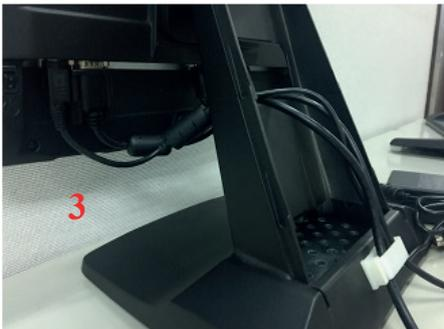
4. Connect the end of D-SUB 9P female of the "D-SUB 9P to DC Jack" cable to the other end of D-SUB 9P male cable
