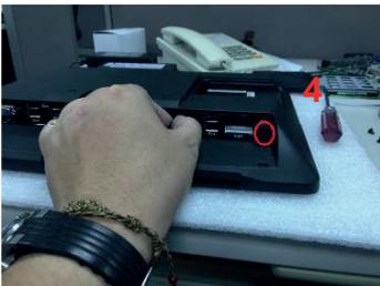
5. Remove the 1 VFD screw
