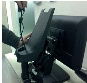
7. Plug in the other end of VGA and DC Jack of the “D-SUB 9P to DC Jack” cables to the 15” 2<sup>nd</sup> display
