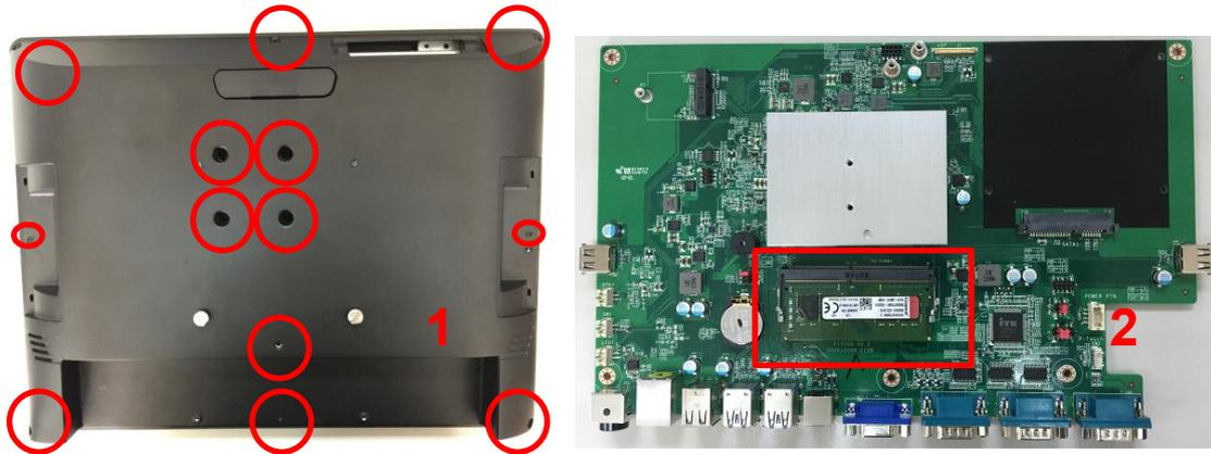
1. Dis-fasten 13 screws and remove the back cover.
