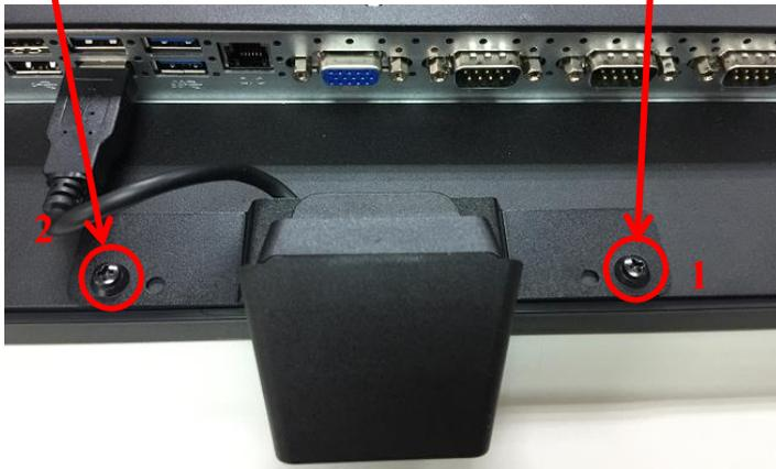
1. Install the barcode scanner with bracket attached by tightening the 2 screws
